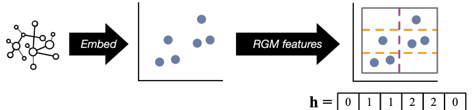
Fig. 1: Overview of our framework. Given an input graph, node representations are learned via an appropriate embedding technique (§ II-B). Our proposed feature mapping RGM then aggregates the graph’s node embeddings in vector space (§ III).
